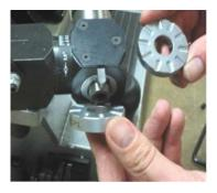
9. Tighten the index plate with the bolt, and return the index knob.
